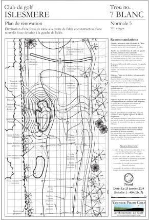
Plan prepared for the removal of a fairway bunker and the construction of a new bunker on the other side of the fairway.
